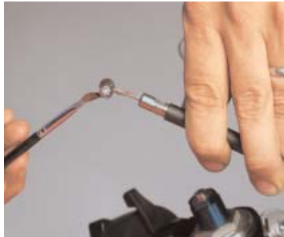
Apply a protective coat of grease to all exposed sections of cables. Don't forget to lube the fittings, so they will move freely within their mounts.
