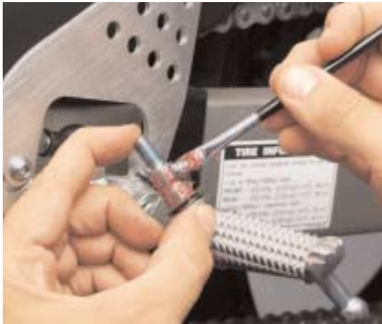
Before lubing pivot points, wipe them clean of any dirt or grit. Keep the threads clean and dry. Retorque the fasteners to the proper spec to keep them from vibrating loose.
