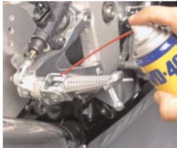
All moving parts, such as peg pivots and side stands, will benefit from a shot of WD-40 or a few drops of oil to keep them working freely. If you're particularly fastidious, you can disassemble the parts and grease them.
