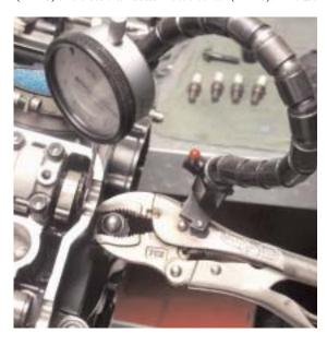
The dial indicator needs to be solidly mounted to the engine. Make sure that the plunger moves parallel to the valve and has enough range to track the valve through its maximum extension.
