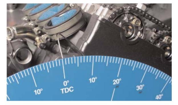
Setting the timing wheel on the crankshaft and mounting a sturdy wire pointer are imperative for accurate cam timing. If you bump the wheel or pointer, you will need to verify TDC before continuing with the project.
